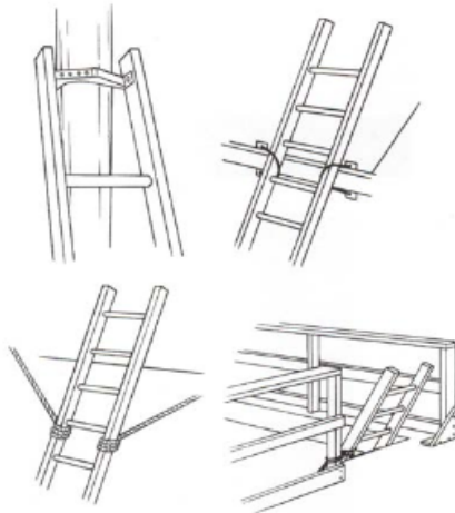
Figure 8.11 Examples of securing a portable ladder at the top
